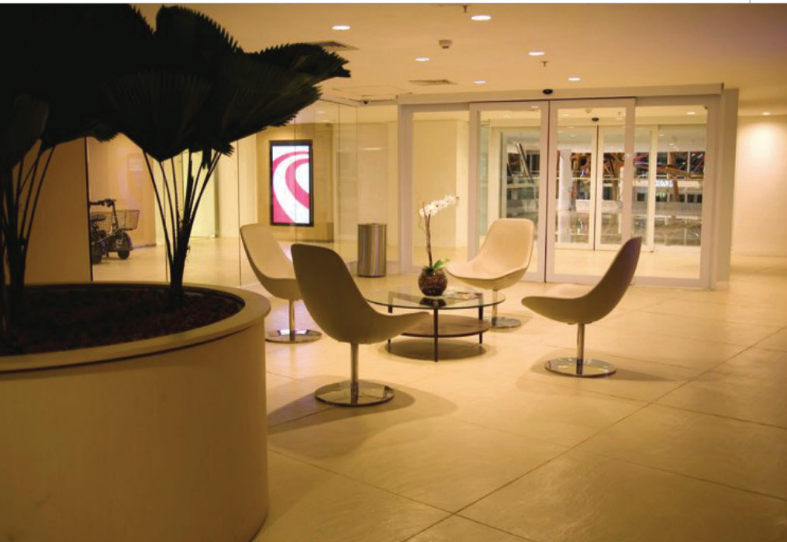
Piso em quartzo Wave Cancun (Santa Margherita S.p.A.) com acabamento acetinado Floor in Wave Cancun quartz (Santa Margherita S.p.A.) with the satin finish
